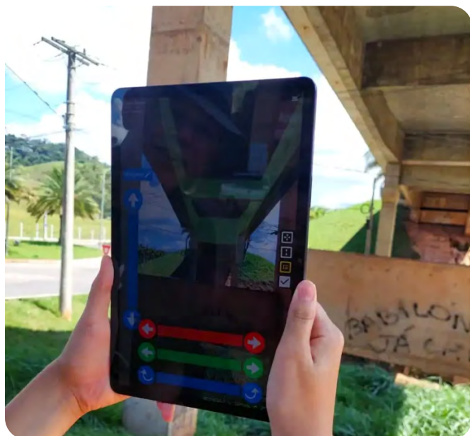
A person holding a tablet Description automatically generated Using GAMMA AR to overlay the BIM model onto the Coimbra I Viaduct for structural inspection. Image courtesy of Universidade Federal de Viçosa (UFV)
